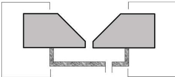
When nominal gas sealing is provided at the ends of the joint seam, a gas pressure is created under the bead that is sufficient to provide protection from contamination and act as support for the molten metal. Inert gas backing produces good root profiles.
