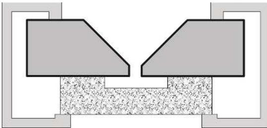
To ensure the bar cannot be welded to the joint, this temporary support often is water-cooled and manufactured from copper.
