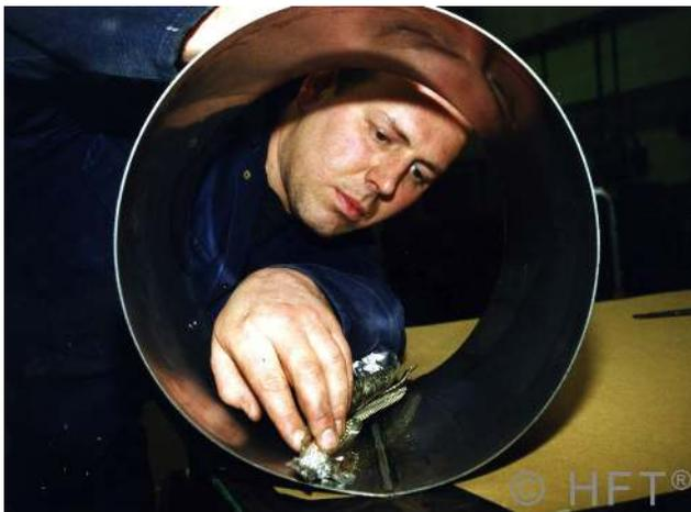
After the welding, the tape is removed from the weld zone by peeling. The tape typically is suitable for use on most common materials such as carbon, alloy, and stainless steels cast iron and copper, nickel and titanium alloys. It is used in conjunction with the MMA,GTAW, GMAW processes.
